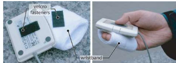
Figure 8. Using a wrist band and Velcro fasteners (left) to secure touchpad in hand (right) while the user is in motion.
